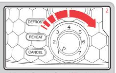
Adjust the Browning Control (3) to the desired setting. Select setting 1 for very light browning from a shorter toasting duration, through to setting 7 for heavier browning over a longer toasting duration.
